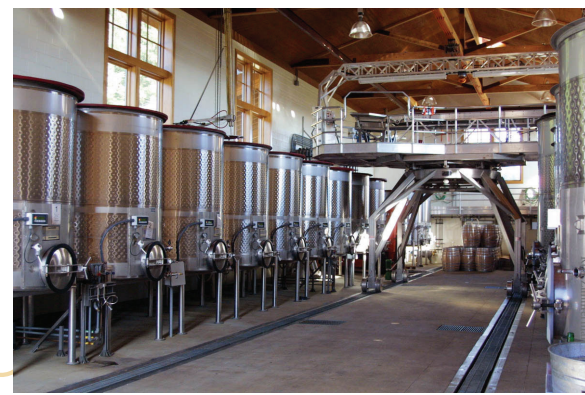
Lemelson Vineyards' fermenters are fed grapes from above by a rolling platform that was designed by Eric Lemelson. The winery is gravity-fed; the vineyards are organic.
